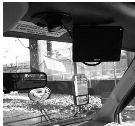
This seven-inch LCD color monitor backup camera system with 30 ft night vision and audio helps increase visibility and awareness.
