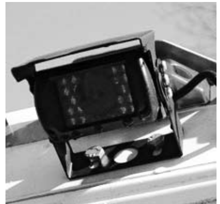
Cameras mounted on the rear outside of the vehicle typically have a dust/water guard.
